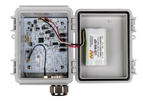
LoRa radio, with support for CANopen available via undertaking a project with Definium.
